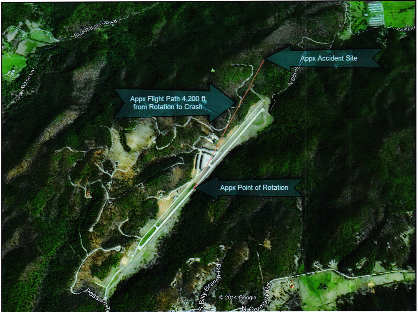
(ABOVE) The aircraft crashed left of the extended centerline approximately three-quarters of a nautical mile from the point of rotation in rising terrain 300 feet higher than the field elevation.
